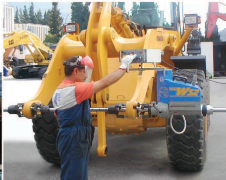
Reconditioning and Realignment of the pin holes of a wheel loader.
