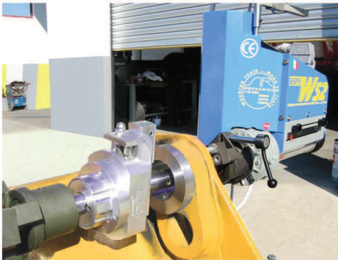
(KIT 2000) Orthogonal machining of external cylindrical surfaces and creation of circlip grooves.
