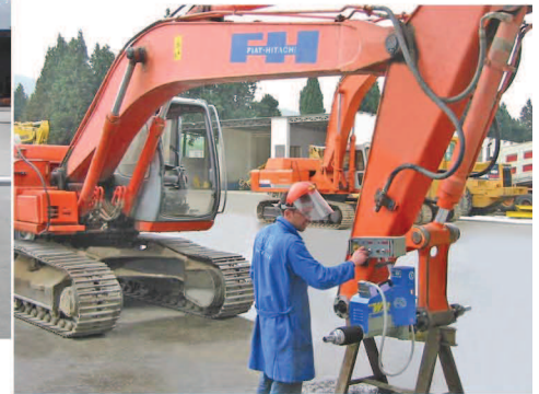
Reconditioning and Realignment of the pin holes of a wheel loader.
